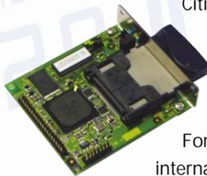
Citizen knows that connectivity is key so the printers have three high performance internal interfaces as standard: a high-speed parallel interface (called an "IEEE1284"), a fast USB interface and an RS232C serial interface operating up to 115,000 bps.
