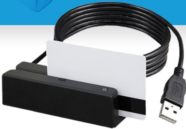
The Element MSR213 Series USB magnetic stripe readers are ideal for retail, time keeping, security and other card reader related applications. The triple tracks of the MSR213 Series are uniquely designed to read credit/debit/loyalty cards and driver licenses, conforming to wide range of standards.
