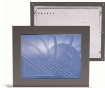
Industrial Flanged Bezel Option (Part number: 29368) 411.0 x 316.9 mm 16.18 x 12.48 inches
